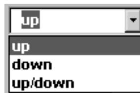
**up** - As the level rises, the continuous level calibration is updated at each point level sensor (capacitance + setback capacitance).
